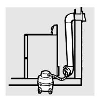
Inspect and clean the dryer exhaust ducting at least once a year to prevent clogging. A partially clogged exhaust can lengthen the drying time. To clean the exhaust duct follow these steps:
